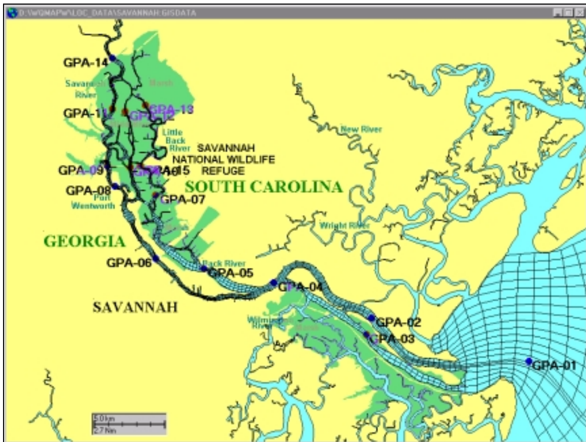
Figure 3 Lower Savannah River Estuary map showing the 1997 long term monitoring stations GPA-01 through GPA-14. The WQMAP boundary-fitted model grid as applied to the estuary is also shown.
